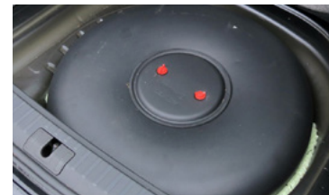
An LPG tank in the floor of the boot
