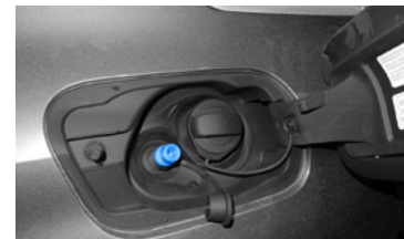
A separate connection on the tank filler neck
