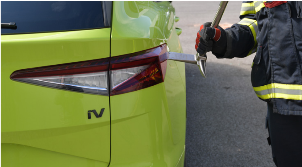
The high-voltage cut-out connection in vehicles manufactured from 2023 is also behind the right rear light
