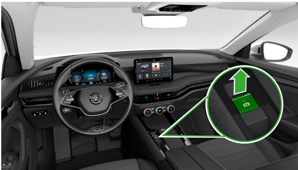
Vehicle with a conventional engine and automatic gearbox: Apply the electronic parking brake or lift the handbrake
