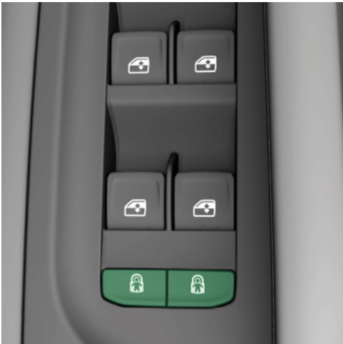
Deactivation of the electric childproof lock using the button in the door trim
