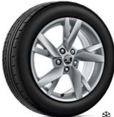
Lyra silver metallic 6.5J × 17" ET46 for 205/55 R17 5E3 071 497E 8Z8 5E3 071 497AC 8Z8*
