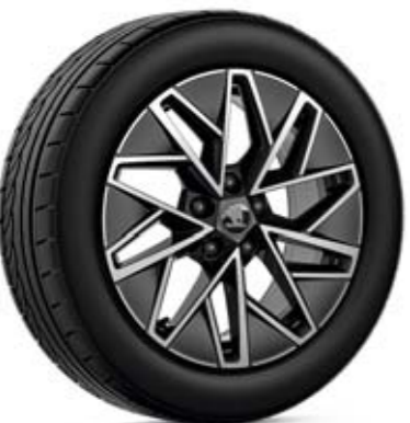
Slagard black metallic, brushed 7.0J × 17" ET46 for 205/55 R17 5E3 071 497D FL8 5E3 071 497AG FL8*
