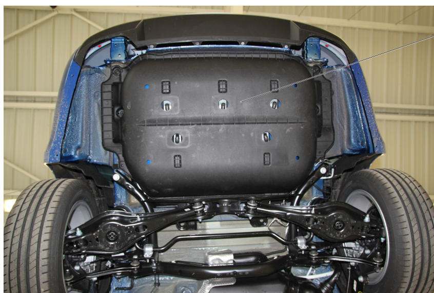
Natural gas tank behind the rear axle
