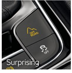
Are you travelling to the mountains or to the wild? Then try the magic OFF-ROAD button. This will switch all assistance systems into an off-road mode – the gas pedal will respond less sensitively, the Hill Descent Control will start braking automatically... allowing you to drive down steep slopes and tackle obstacles without any problems.
