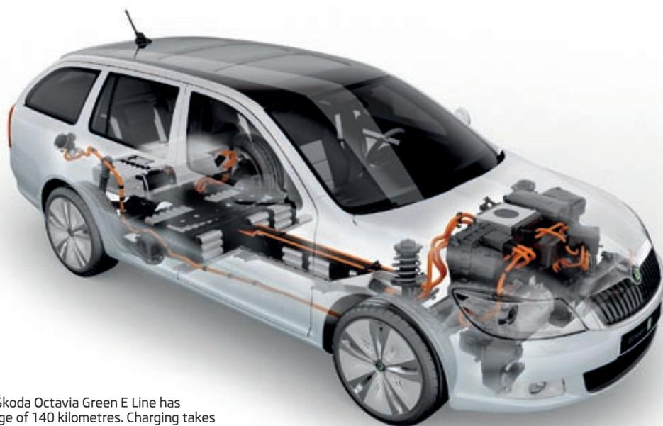
The Škoda Octavia Green E Line has a range of 140 kilometres. Charging takes about four hours with a 400-volt power current and eight hours with a standard household voltage of 230 volts.
