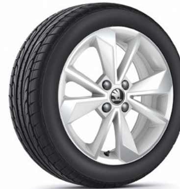
SCORPIUS 1ST 071 496N FM9 light-alloy wheel 6.0J x 16" ET43 for 185/50 R16 tyre white, brushed
