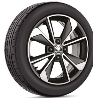
SCORPIUS 1ST 071 496J FL8 light-alloy wheel 6.0J x 16" ET43 for 185/50 R16 tyre black metallic, brushed
