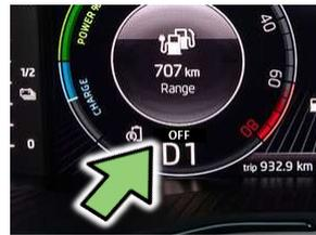
The electric engine is noiseless. The display in the combi (Powermeter) shows message whether the electric drive is switched off "OFF" or ready for operation "READY".
